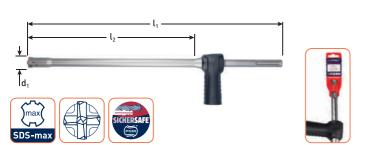
Execution: Dust-free drill bit with SDS-max shank (ø18mm) and integrated dust-extraction. PGM certified three-pieced carbide insert with two cutting edges and special centering tip, made of high-grade alloyed steel and carbide with the latest and unique geometries.
