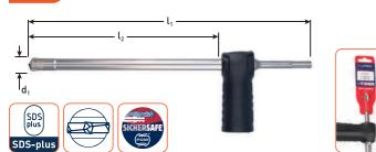
Dust-free drill bit with SDS-plus shank (ø10mm) and integrated dust-extraction. PGM certified one-piece solid carbide insert with two cutting edges and special centering tip, made of high-grade alloyed steel and carbide with the latest and unique geometries.
